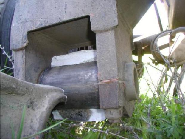
*Hopefully this picture of a broken walking beam will come out. On the bottom you can see the darker area where it had been broken for a time until it completely let go, leaving the log truck and it's load in the ditch.*
