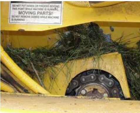
Fig. 2: Clear combustible debris in forestry equipment as it accumulates, even several times a day.
