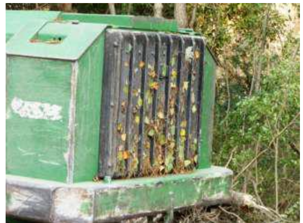
Blocked radiator can cause overheating, leading to fire.
