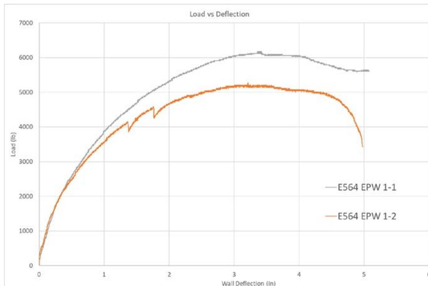
**Figure 3. Shear Load Deflection Curves: E564 Test - Baseline EP&B Walls**
