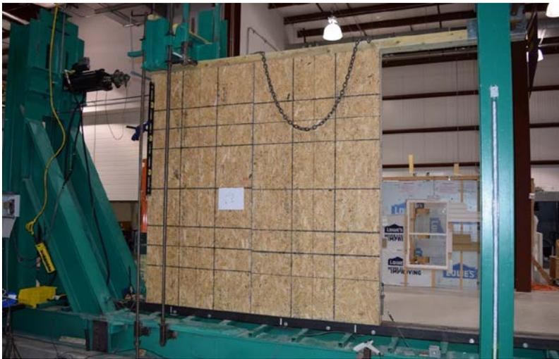
Figure 1. Reference Wall in Testing Apparatus Prepared for ASTM 72 Test
