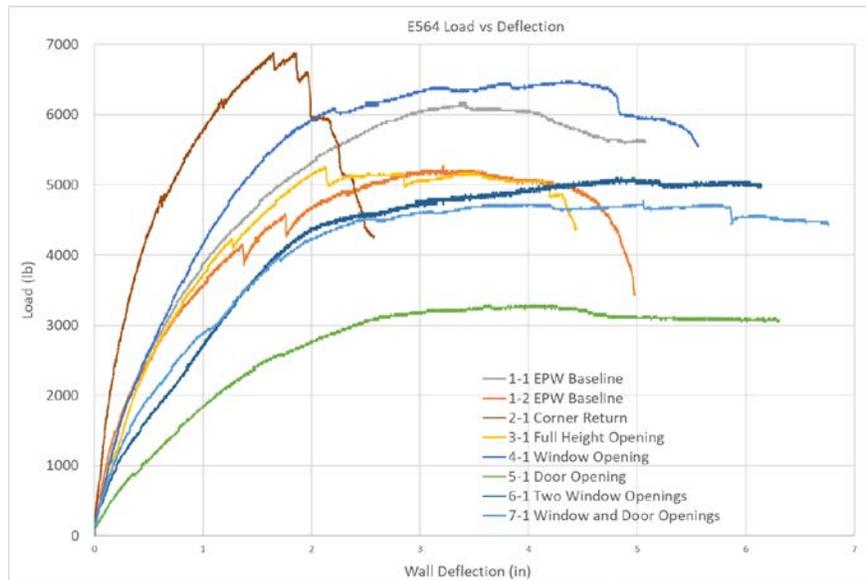
Figure 4. Load Deflection Curves: E564 Test – EP&B Walls
