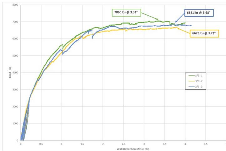
**Figure 2. Maximum Loads: E72 Test - EPW Baseline**
